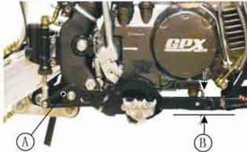
A. Rear Brake Pedal B. 20 ~ 30mm (0.8 ~ 1.2 in)
