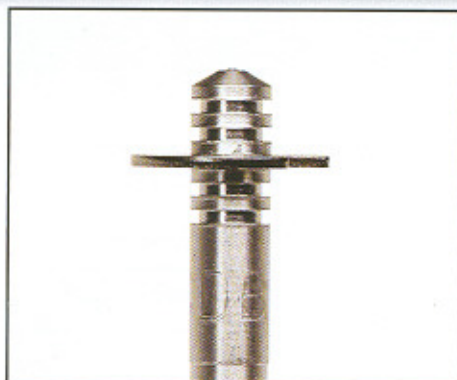
Location of C-clip on jet needle determines mid-range fuel mixture.
