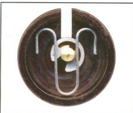
Be sure the V-shaped jet needle retaining clip is in place and will hold the jet needle securely in the slide.
